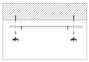
1. Fix the ceiling plate to the ceiling with plugs and screws suitable for your ceiling type.
