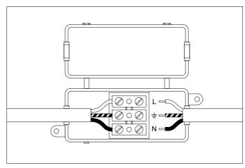
**3.** Connect the 3 wires according to their colours. Brown is the live wire (L), blue is the neutral wire (N), green/yellow is the earth wire  $(\frac{\bot}{-})$ .
