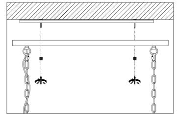
$\textbf{4.}\,\text{Place}$  the canopy over the ceiling plate and fix it with the nuts.
