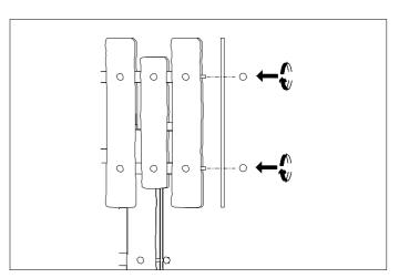
6. Alternately fix the glass to the frame with the screws supplied.
