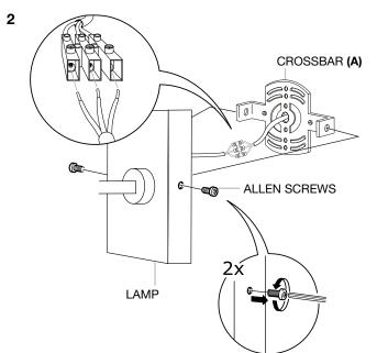
Turn off the electricity supply at the main circuit panel before installing. Do not connect the electricity supply until your luminaire is fully assembled and installed.
