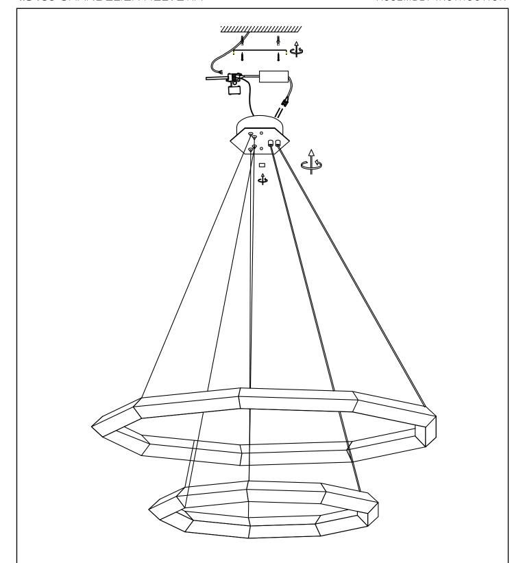
Fix the crossbar to the ceiling by using mounting plugs and screws suitable to your ceiling type.
