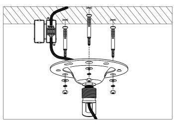
1. Fix the ceiling bracket to the ceiling by using mounting plugs and screws suitable for your ceiling type. Connect the 3 power wires. Brown is the live wire, blue is the neutral wire, green/yellow is the earth wire.
