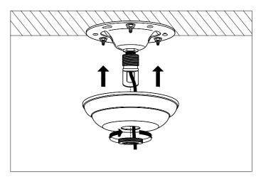
2. Slide the canopy over the ceiling bracket and fix it with the retaining nut.
