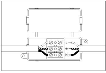
2. Connect the 3 wires according to their colours. Brown is the live wire (L), blue is the neutral wire (N), green/yellow is the earth wire ( $\frac{1}{m}$ ).
