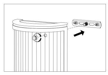
3. Slide the lamp over the crossbar and tighten the knob until the lamp is secure.
