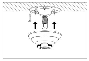
2. Slide the canopy over the ceiling plate and fix the retaining nut.
