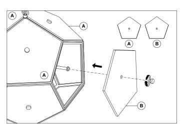
**6.** Fix the alabaster sheets with the screws supplied. Place the 3 top alabaster sheets (A) and the the bottom alabaster sheets (B).
