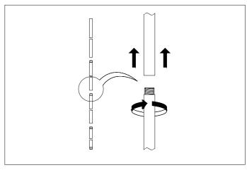
2. Determine the desired height of the lamp and use either one, two or three of the pipes supplied. Thread the wires through the pipe.
