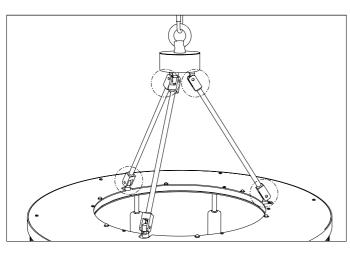
1. Connect the two pipes to the lamp and to the ceiling canopy as shown.
