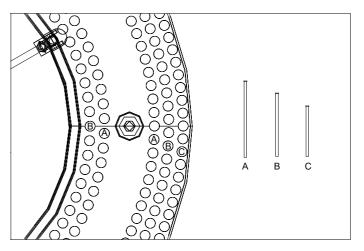
6. Place the glass according to the schedule, from inside out: B, A, A, B, C. After placing the glass, place the plate back.
