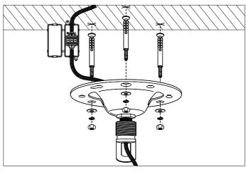
2. Fix the ceiling bracket to the ceiling by using mounting plugs and screws suitable for your ceiling type. Connect the 3 power wires. Brown is the live wire, blue is the neutral wire, green/yellow is is the earth wire.
