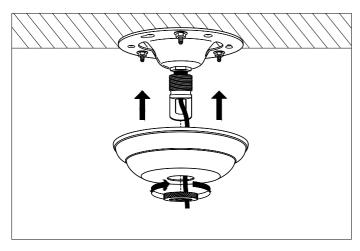
3. Slide the canopy over the ceiling bracket and fix it with the retaining nut.
